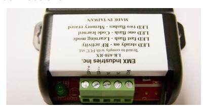
15 FIFO register (code 16 will delete first code put in) 3.125" x 2.563" x 1.0" (80mm x 65mm x 25mm)
